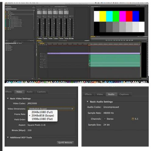
The resulting DCP was tested using the Wraptor player from Quvis at SAWVideo in Ottawa, an artistrun not-for-profit media centre. As the screen capture shows below, the resulting DCP includes a 5.1 audio track
